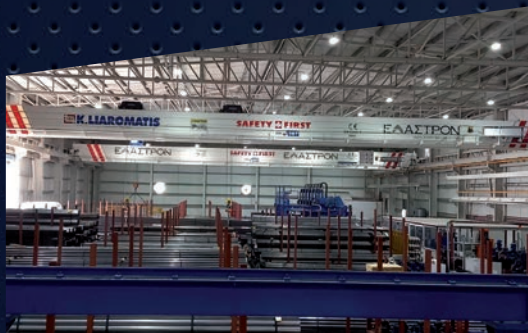
2 units, 12 t x 30.8 m, 12.5 t x 31 m & 2 units, 8 t x 30.8 m, with Verlinde lifting equipment. Client: Elastron 2022, Aspropyrgos, West Attica
