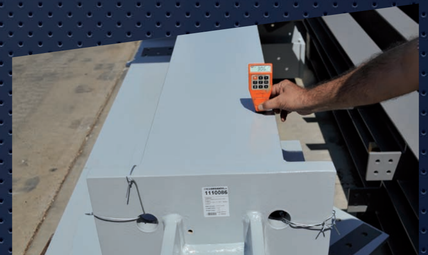
Paint Thickness Inspection
