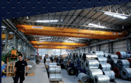
32 t, 25 t & 20 t x 28.65 m, with Verlinde lifting equipment. Client: Sidma Steel 2007, Oinofyta, Boeotia
