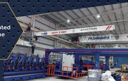
1.6 t with Verlinde lifting equipment. Client: Elastron 2023, Aspropyrgos, West Attica
